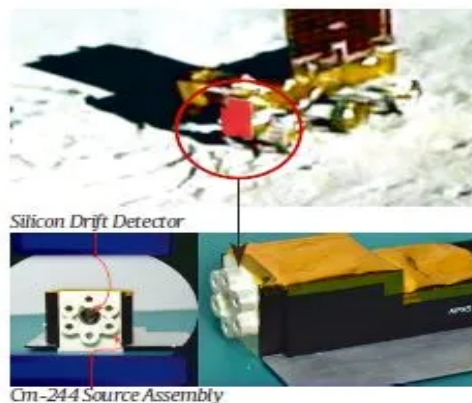
(Top) Chandrayaan lander as seen by rover; the APXS instrument. ISRO
