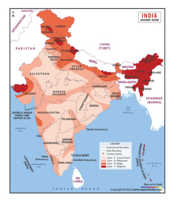
According to the revised IS 1983-2002 seismic code, seismic zones are **mapped** to a modified CIS-64 scale, an alternative to the MMI scale for seismic zoning.
