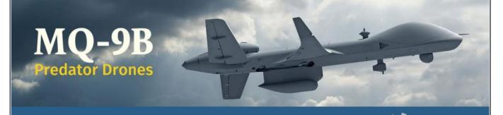
Max Gross Takeoff Weight: 5,670 kg Fuel Capacity: 2,721 kg Payload Capacity: 2,177 kg across 9 hardpoints (8 wing, 1 centerline)
