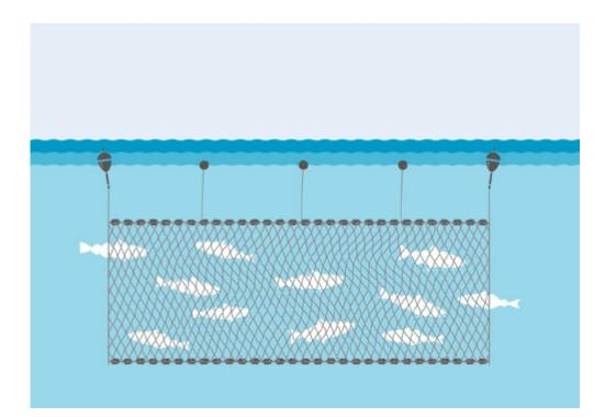
• **Bull trawling** - In bull trawling or pair trawling, a net is tied between two mechanised boats and it is dragged for some kilometres to catch fish.
